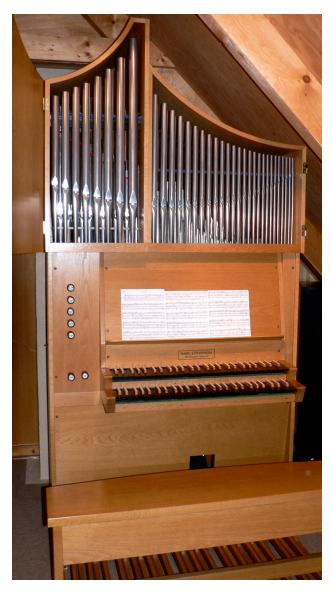
This small organ has two manuals, 56 keys, and a pedal of 27 keys. There are only 5 stops, with 27 common bass pipes for the three keyboards. However the pedal has its own wind chest, then available air channels. The ergonomics, often a weak point of positives, is excellent: large music stand not too close to the eyes, front pipes
